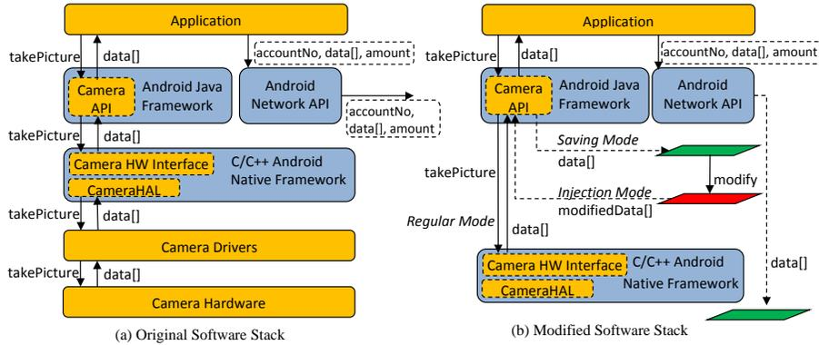
Fig. 4: The Original and Modified Camera Subsystems
