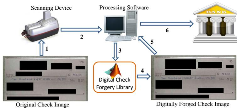
Fig. 1: Check Truncation System and Attack Description
