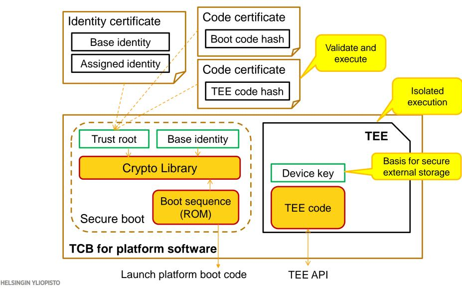
Authorized execution of arbitrary code, isolated from the OS; access to device key 11
