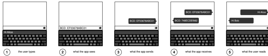
Fig. 1. The BabelCrypt system at work. The user types a message (1), when pressing send the keyboard encrypts the message and passes it to the application (2). The application sends the message (3). The application receives an encrypted message (4) and the overlay decrypts and displays the message to the user (5). Stages 3 and 4 are transparent to the user.
